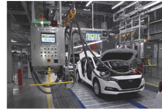
Coolant Filling Equipment
